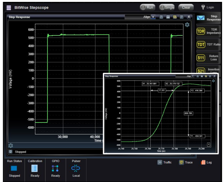
Step Response View; Inlay: 10/90 Step Response Rise Time
