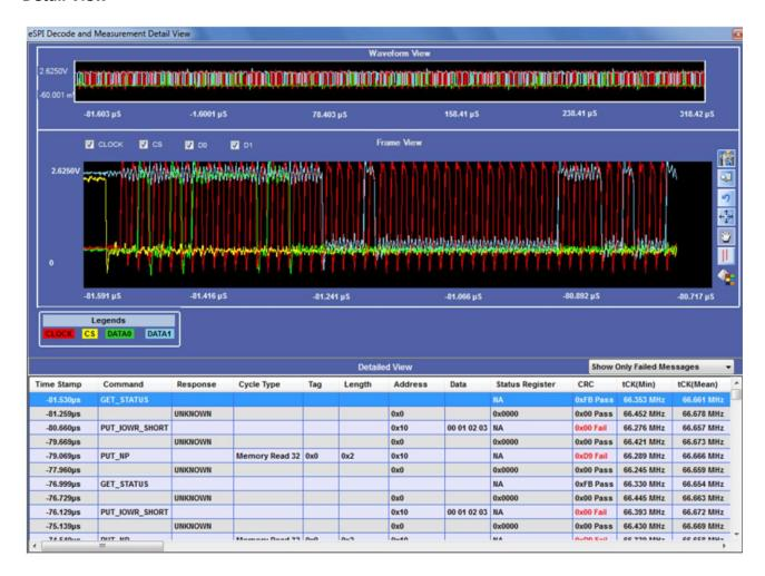
Once the electrical failure or protocol problems needs to located specific protocol packets to debug the design issues. In Detail view, the acquired waveform is plotted. The waveform plot is linked with the packet being displayed on the grid. The plot contains various features like zoom, pan and cursors. By linking specific protocol packet to electrical waveform, engineers can quickly locate root cause of the problems.
