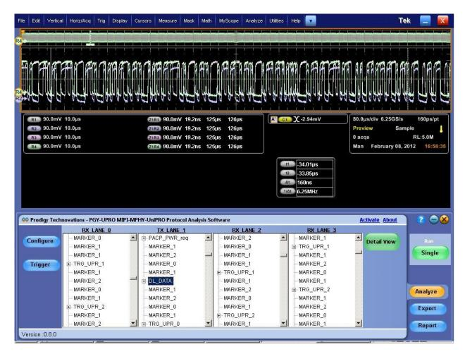
PGY-UPRO/LLI/UFS runs inside the Tektronix oscilloscopes and decodes protocols and displays the decoded data of multiple lanes. This software links the decoded data to the electrical signal in the oscilloscope display. UniPRO/LLI Protocol-based trigger can be set up using the built-in high speed serial trigger capabilities in Tektronix oscilloscopes.
