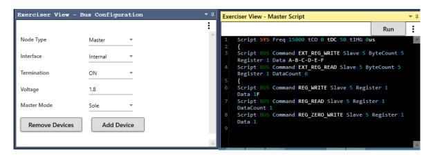
PGY-SPMI-EX-PD supports SPMI traffic generation using GUI and Script. User can generate simple traffic generation using the GUI to test the DUT. Script based GUI provides flexibility to emulate the complete expected traffic in real world including error injections. In this sample script user can generate SPMI traffic as below.
