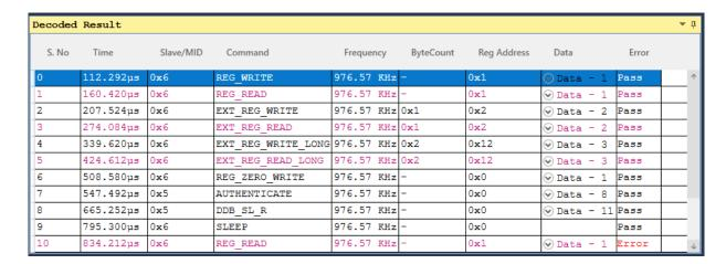
Protocol window provides the decoded packet information in each state and all packet details. Selected frame in Protocol listing window will be auto correlated in timing view to view the timing information of the packet.
