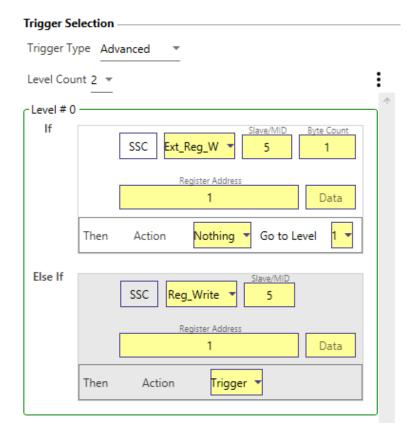
PGY-SPMI-EX-PD supports simple trigger capabilities. Analyzer can trigger on any of the Protocol packets such as Reg Write, SLEEP or WAKE UP. Advanced Trigger provides the flexibility to monitor Multiple trigger conditions and can set multiple state trigger machine. User can initiate a timer and trigger on set timer values.
