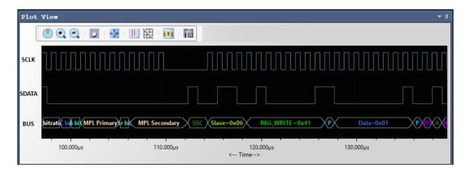
Timing view provides the plot of SCL and SDA signals with bus diagram. Overlaying of Protocol bits on the digital timing waveform will help easy debugging of Protocol decoded data. Cursor and Zoom features will make it convenient to analyze Protocol in timing diagram for any timing errors.
