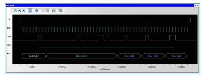
Timing view provides the plot of CS, CLK, DQO and DQ1 signals with bus diagram. Overlaying of Protocol bits on the digital timing waveform will help easy debugging of Protocol decoded data. Cursor and Zoom features will make it convenient to analyze Protocol in timing diagram for any timing errors.
