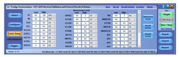
Configure panel helps in selecting the Signal Source, Such as Channels, Wfm Files and CSV Files (Digital). Live Analog or Digital Channels of the oscilloscope can be used for analysing the signal. The software decodes the data and displays both the protocol data and electrical measurements as shown below. Offline analysis is made using the stored .wfm files (Analog channels data) or from csv file (Digital Channel data)
