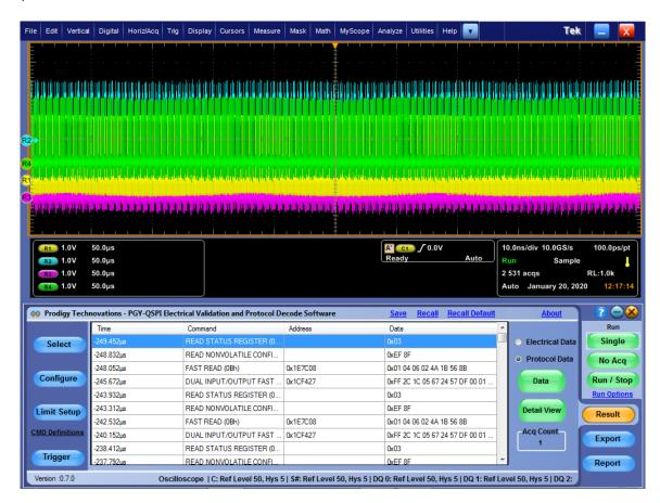
In detail view links the selected command to electrical waveform for easy debugging of protocol related problems
