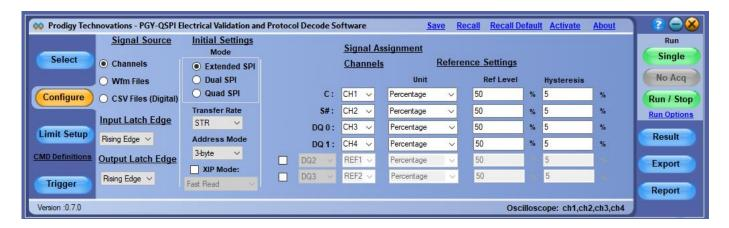
*Limit Setup* tab helps to set up the limits and reference levels of each selected measurements. In order to characterize and validate QSPI signals PGY-QSPI software provides graphical measurement reference level setup to set measurement reference level of QSPI signals.
