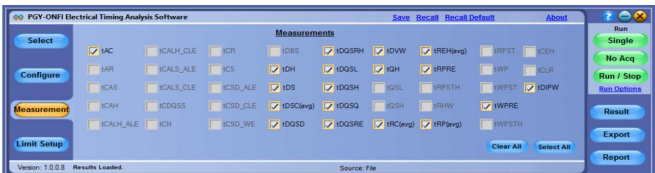
Result View lists all electrical measurements with pass/fail report
