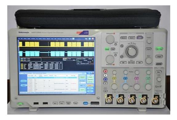
PGY-I3C Software installed in Tektronix oscilloscopes can be launched by clicking on PGY-I3C icon in oscilloscope desktop folder. Now user has simultaneous view and control to oscilloscope as well as PGY-I3C Software. User can analyze I3C in single acquisition mode, Repetitive mode and as well as No Acq mode. In No Acq Mode, I3C software analyses already captured I3C signal that is present in the acquisition memory of the oscilloscope.
