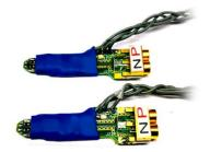
P5021-L-WE 14 Gbps probe tips with passive equivalizer at input
