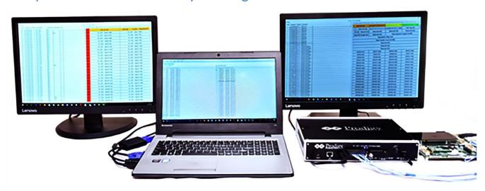
PGY-UFS 4.0-PA UFS Protocol Analyzer provides USB 3.0 interface for host computer connectivity. High-speed host connectivity enables continuous streaming of protocol data to host HDD and storage for long period of time. Software offers multi-view such as MPHY view, UniPro view and UFS View. Each view lists the respective protocol packets and its details with correlation of each layer for easy debug.
