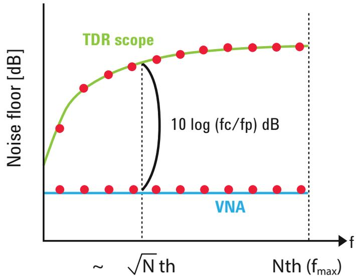
Figure 10. Comparison of dynamic range of the VNA and oscilloscope in the frequency domain.
