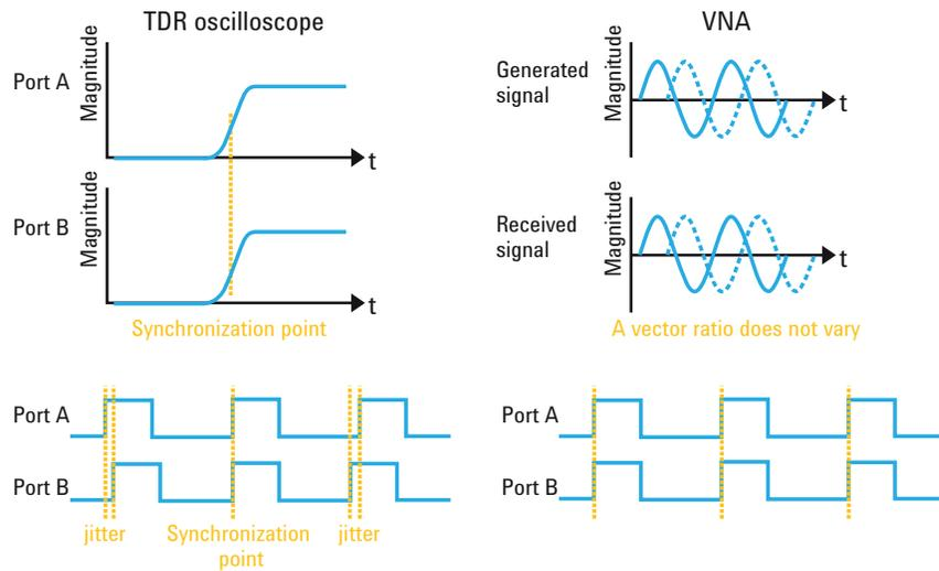
Figure 12. Time synchronization of multiple sources on the TDR oscilloscope (left). Adjusting for phase delay on the VNA for time synchronization (right).
