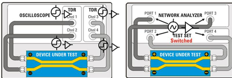
Figure 11. Block diagram of stimulus settings on the TDR oscilloscope (left) and VNA (right) when measuring multiport devices.
