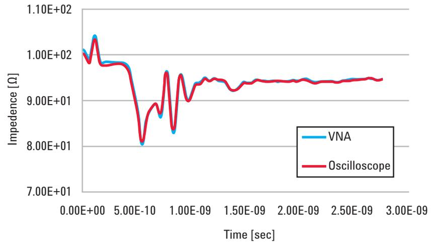
Figure 6. Correlation between measurements taken on a VNA (E5071C) and TDR oscilloscope (86100C) (averaging = 16 is applied to the TDR oscilloscope measurement).
