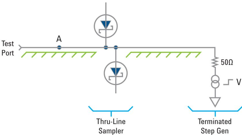
Figure 13. Block diagram of connection between the sampler and pulse generator on a TDR oscilloscope.
