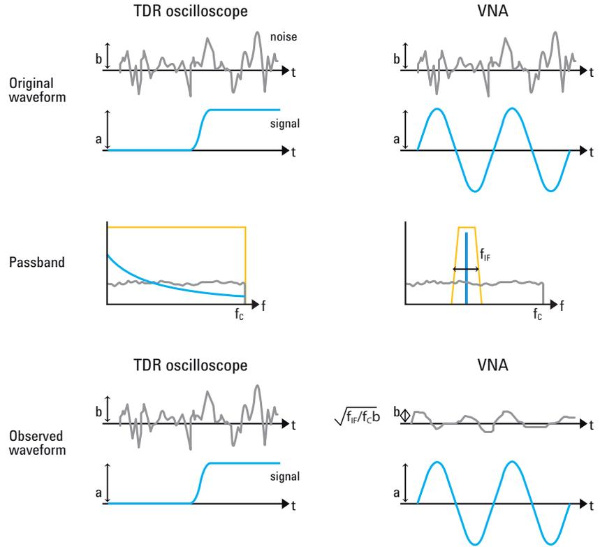
Figure 7. Noise reduction mechanism on the VNA.
