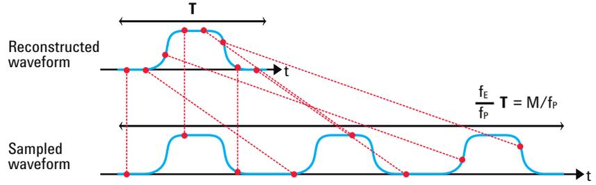
Figure 8. Relationship between the reconstructed waveform and measurement time on a sampling oscilloscope.
