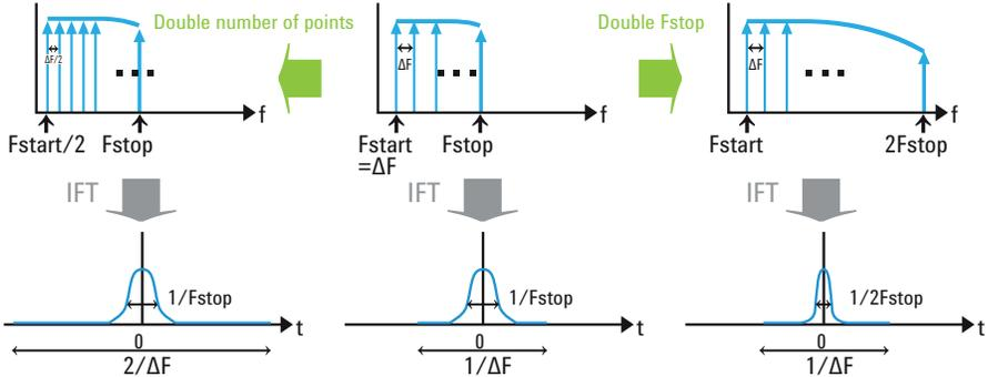
Figure 5. Relationship between the time domain parameters (time resolution and measurement time) and frequency domain parameters (maximum frequency and frequency step).
