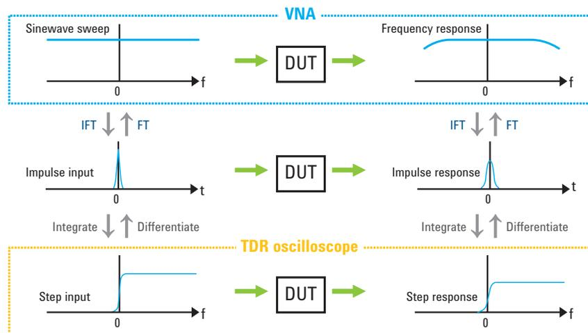
Figure 4. Relationship between the step and impulse response derived from the inverse Fourier transform.
