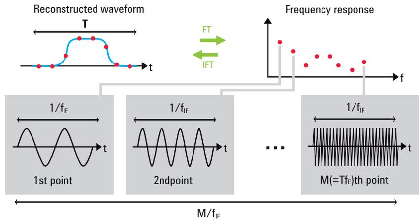
Figure 9. Relationship between the reconstructed waveform and measurement time on a VNA.
