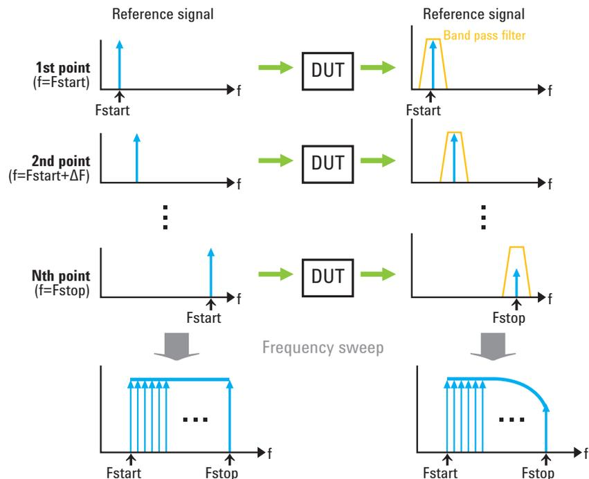
Figure 3. Sine wave stimulus signal is swept across frequency to obtain the frequency response on the VNA.
