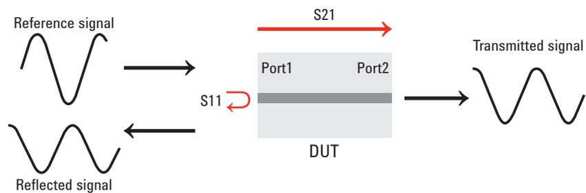
Figure 2. Diagram of reference, reflection, and transmission signals.
